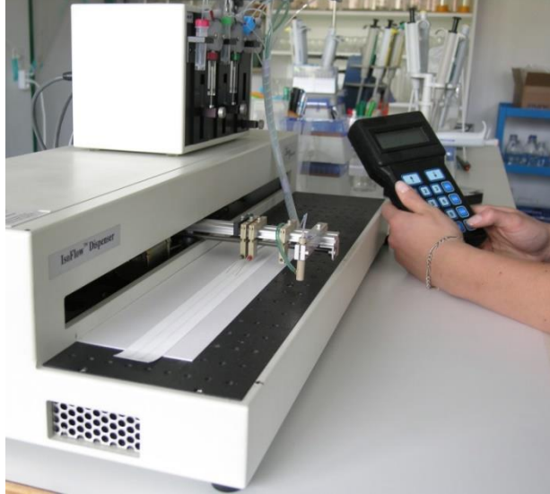
Coating antibodies to the membrane
